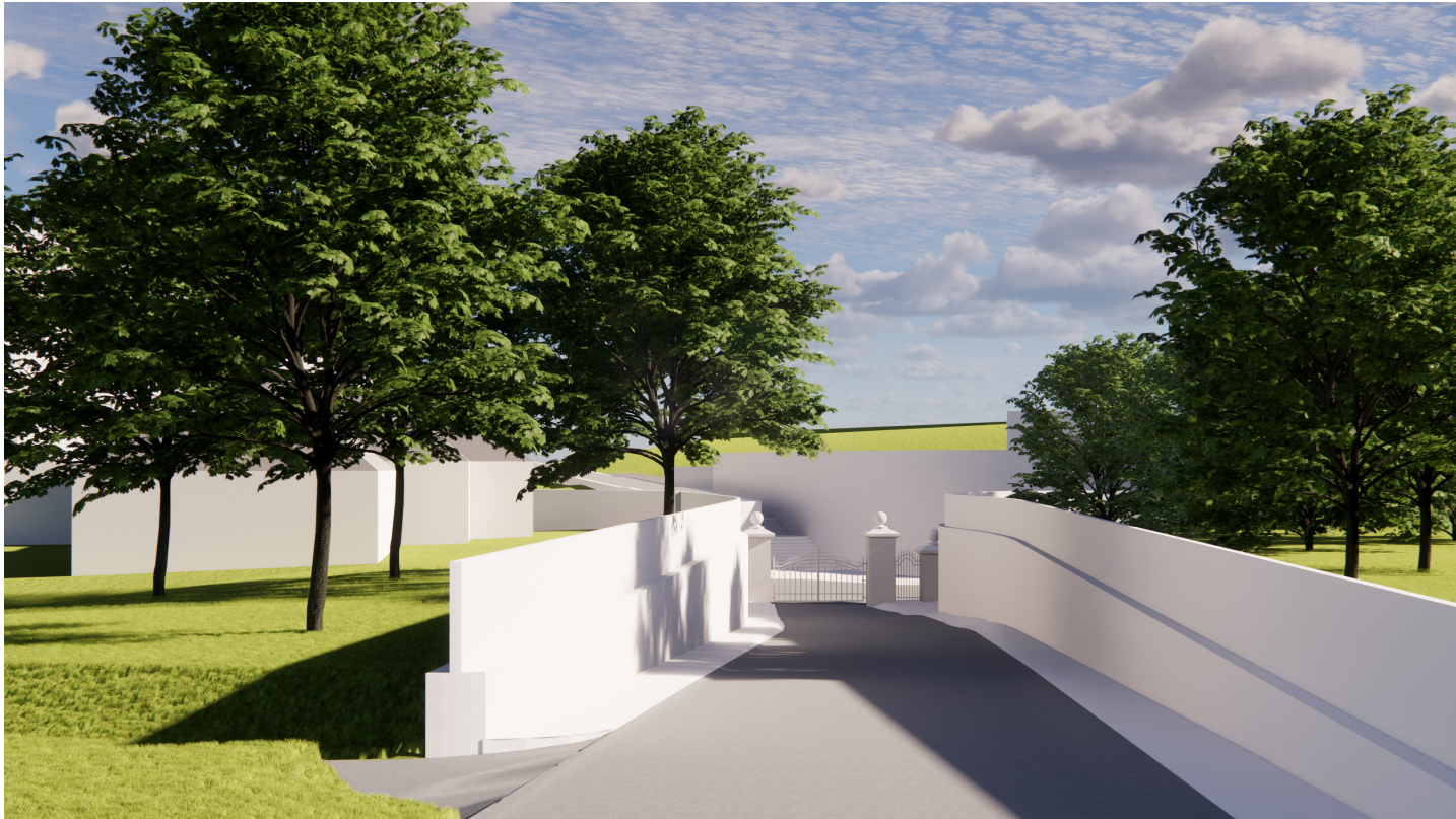
3d view of Ashton House entrance from Ashtown Road (Iarnrod Eireann Proposal) As the level of the Ashtown Road Upgrade, where it meets the existing entrance area, is c. 2.7 metres below existing levels, the Iarnrod Eireann proposal includes a new access road within the grounds of Ashton House, which is a ramped road of c. 45 metres in length, at a gradient of c. 1:20. The proposed new access road will require retaining walls to both sides. The visual impact of the new access road is shown in the above image - the new access road effectively divorces the gatehouse from the entrance sequence, as it is positioned at a different level, and will be visually separated by the access road and its surrounding retaining walls and fence.
