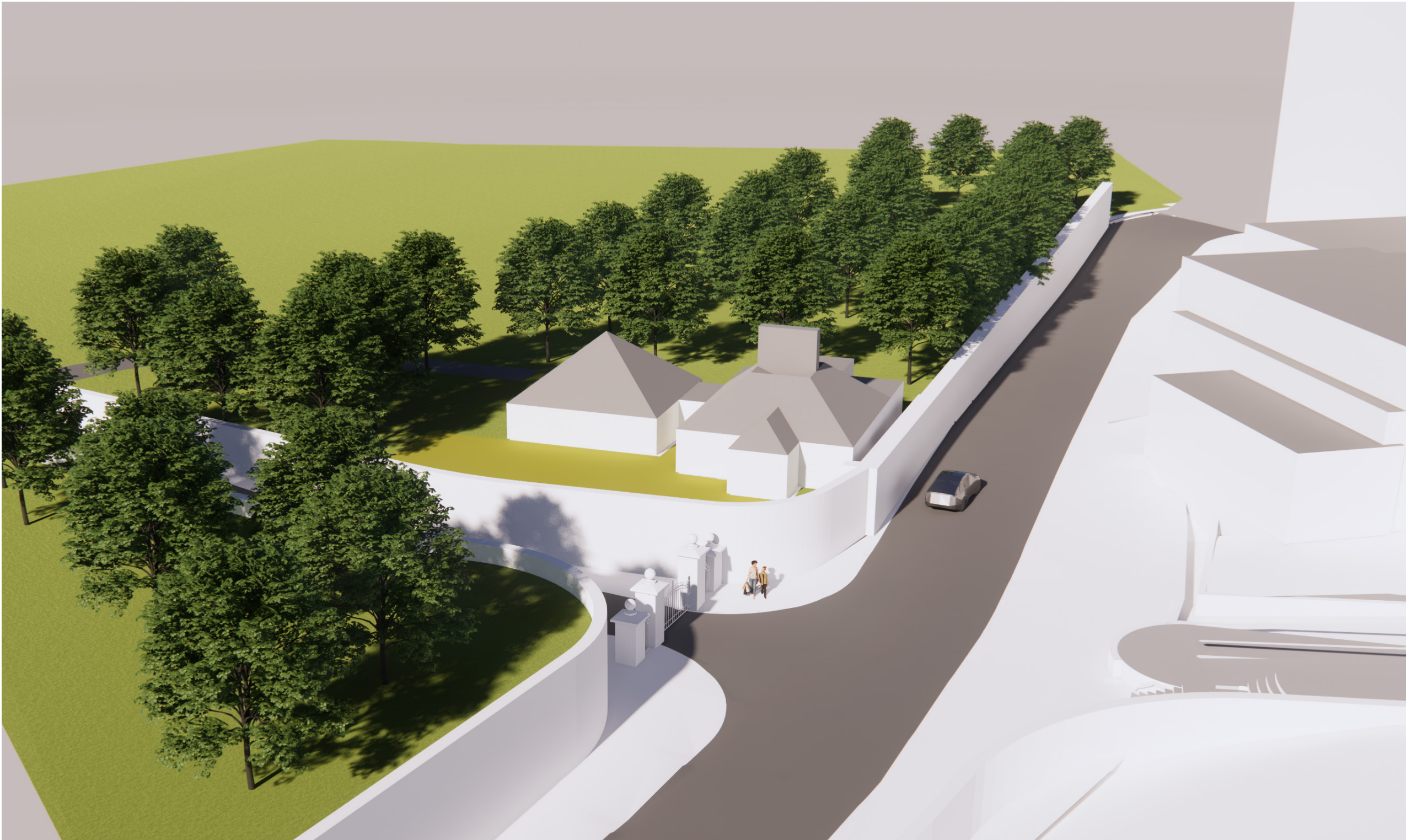
Proposed Ashtown Road Upgrade & Ashton House entrance by Iarnrod Eireann, with change in ground level of c.2.7metres at the existing entrance to Ashton House. As can be seen in the 3d model, the stone piers and gates are dwarfed by the scale of the retaining walls required by the Ashtown Road Upgrade, and the relationship between the stone piers & gates and the Gatelodge is severed.
