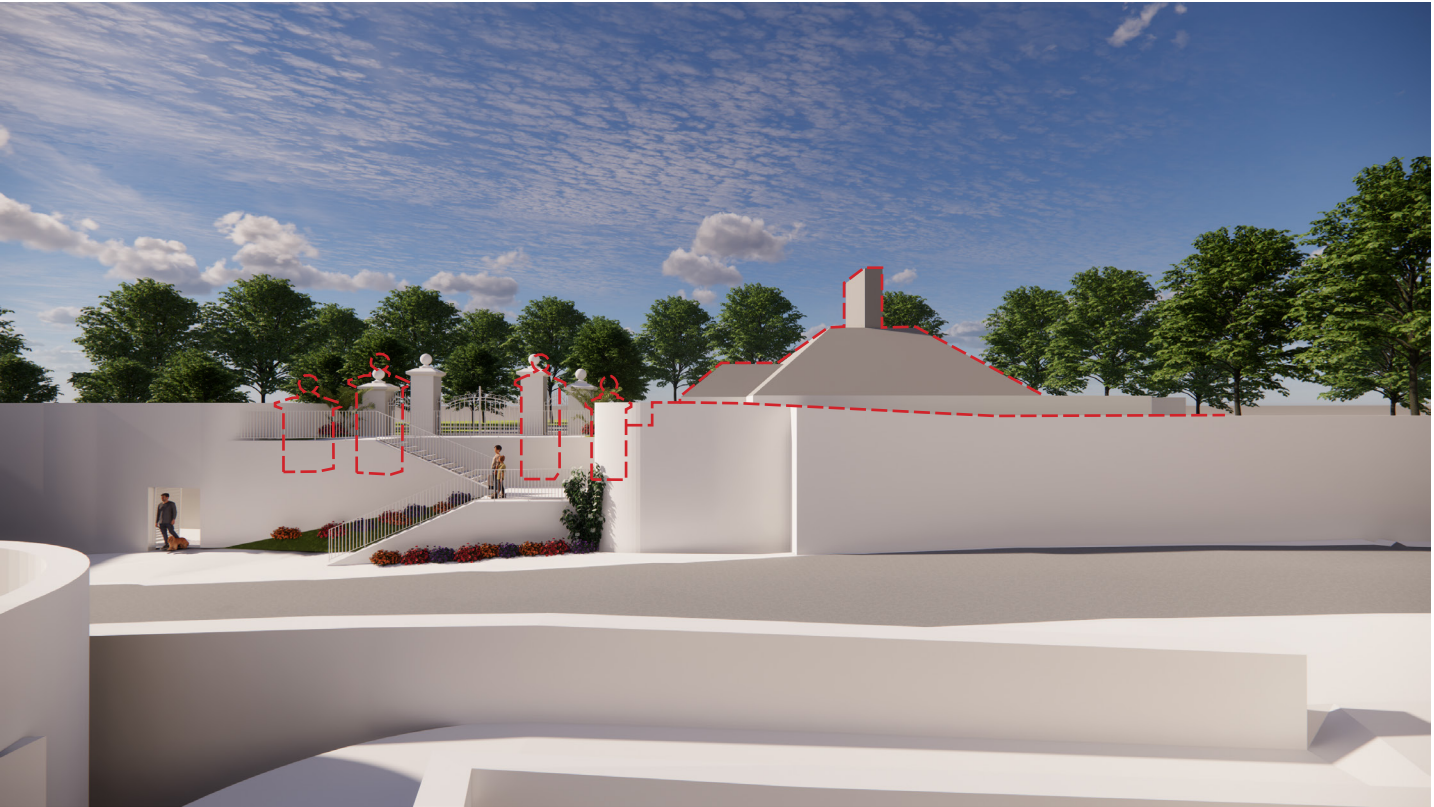
3d view of Ashton House entrance from Ashtown Road (CastlethornProposal) The stone piers & gates (Protected Structures) are removed from their existing position and rebuilt as shown - their position aligns with the western wall of the gate lodge, and their ground level is the same at their existing ground level. The new position of the stone piers and gates creates a “bell mouth” area, where steps and planting are located, which facilitates pedestrian movement between Ashton House and the Ashtown Road Upgrade. A new boundary wall, which forms the western edge of the Ashtown Road Upgrade, with estimated heights of between 4.0 - 5.0 metres, acts as a retaining wall to the Ashton House Lands - the position of the proposed steps and planting screens the height of the boundary walls, mitigating the visual impact of their height.
