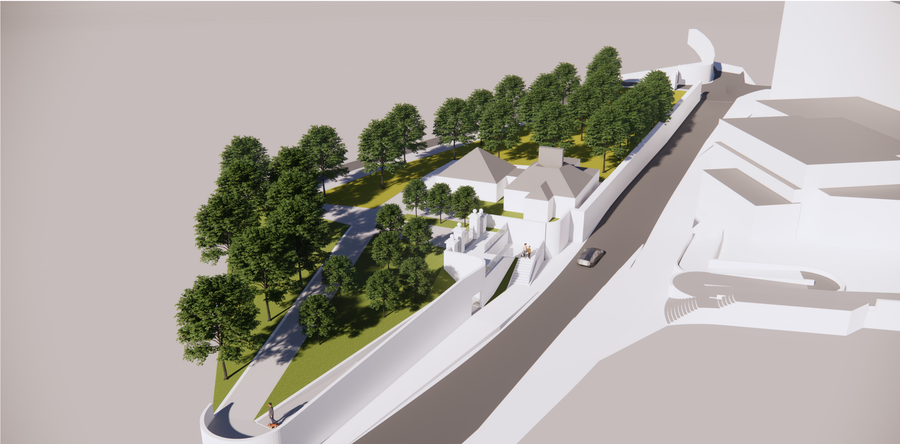
Alternative entrance design to Ashton House by Castlethorn, with the stone entrance piers retained at their existing ground level, and new steps and ramp to negotiate the 2.7m level change. This proposal does not require any changes to the alignment or levels of the Iarnród Éireann design for the Ashtown Road Upgrade.
