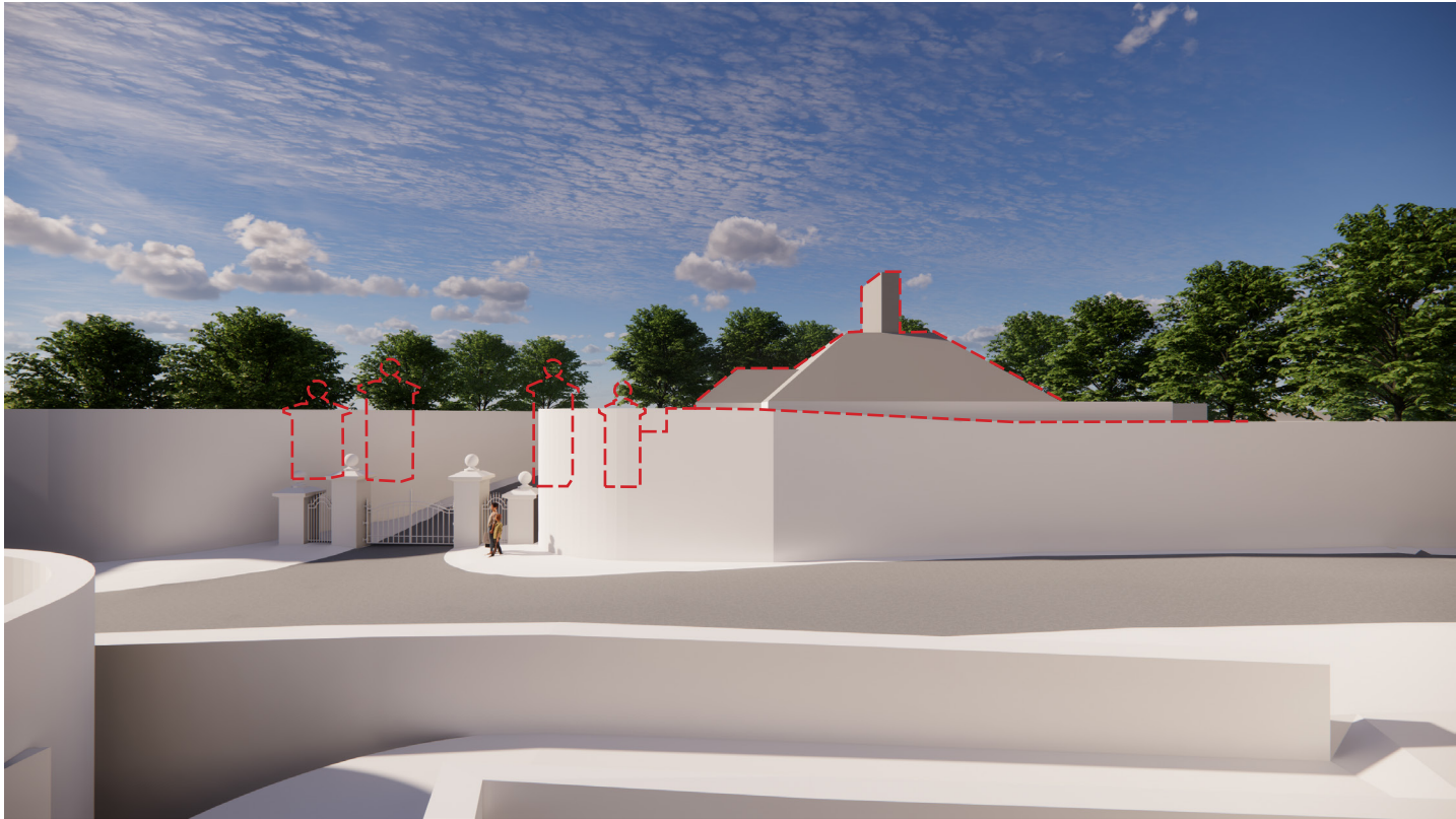
3d view of Ashton House entrance from Ashtown Road (Iarnrod Eireann Proposal) The stone piers & gates (Protected Structures) are removed from their existing position and rebuilt as shown, at a level c. 2.7metres below their existing position. A new boundary wall, which forms the western edge of the Ashtown Road Upgrade, with estimated heights of between 4.0 - 5.0 metres, acts as a retaining wall to the Ashton House Lands. Vehicular and pedestrian access to Ashton House is via the repositioned gates, and the new, steeply sloped access road that would be required within the Ashton House Lands is visible through the gates. Retaining structures will be required on both sides of the new access road to Ashton House, which will create a “tunnel” effect, and overshadowing on the access road.
